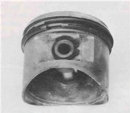
Beemer pistons, made either by Mahle or Kolben Schmidt, use external pin retainers and three rings.
