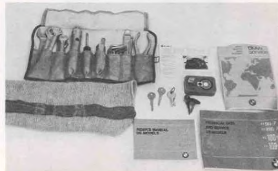
This is all the stuff that's under the seat: tools, a rag, keys, tire patch kit, service and owner's manuals.
