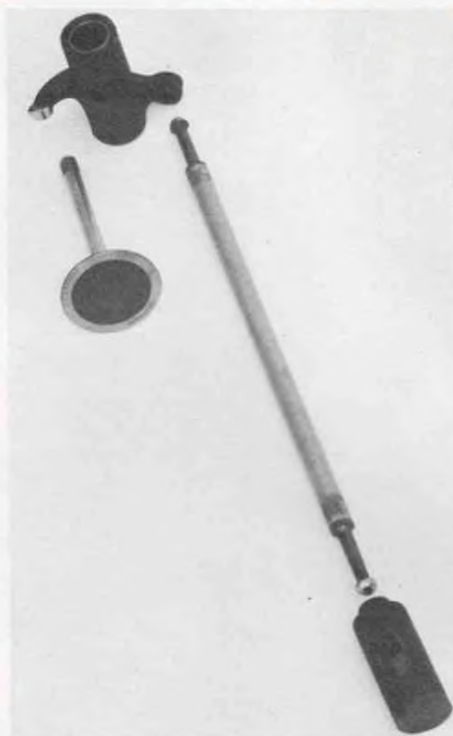
Valve train (left): tappet, pushrod, rocker arm and valve. It's just as simple when it's assembled (below).
