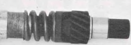
Power from the clutch is transmitted to the gearbox with this shock-absorber-equipped input shaft.
