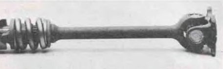
The RT's all-new shock-equipped driveshaft cushions rear end and gearbox, and helps gear disengagement.
