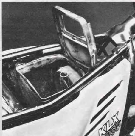
The air cleaner is easy to service; the air box, with its top breather, is almost completely waterproof.
