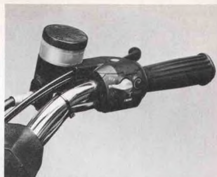
Due to beneath-the-tank space requirements, BMW moved the front brake reservoir atop the handlebar.
