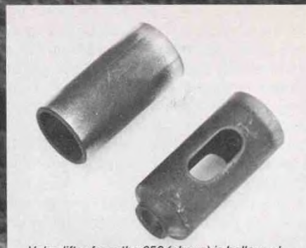
Valve lifter from the 650 (above) is hollow, allows long pushrod length to be maintained.
