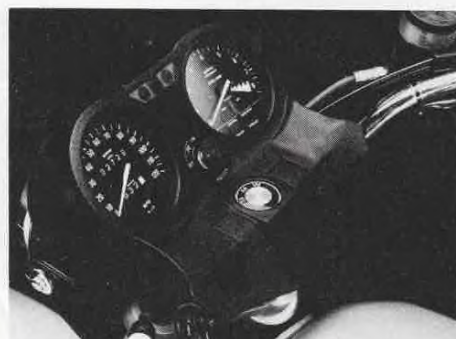
Tach warning light flashes when the 7500-rpm redline is violated. Quartz-halogen headlight is excellent.
