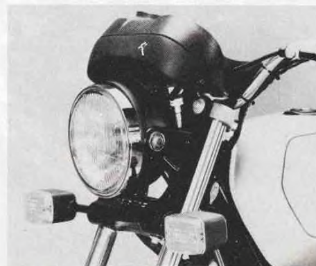
Tach warning light flashes when the 7500-rpm redline is violated. Quartz-halogen headlight is excellent.
