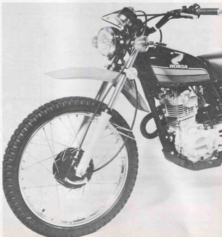
Completely orthodox technical features include a center-axle fork, two-valve head and five-speed transmission.
