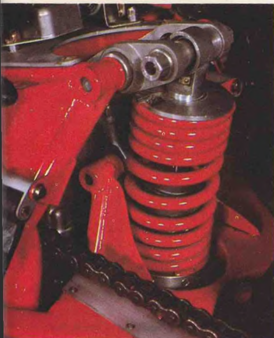
Bottom of shock attaches directly to swing arm; the top is linked to it through an aluminum rocker arm.
