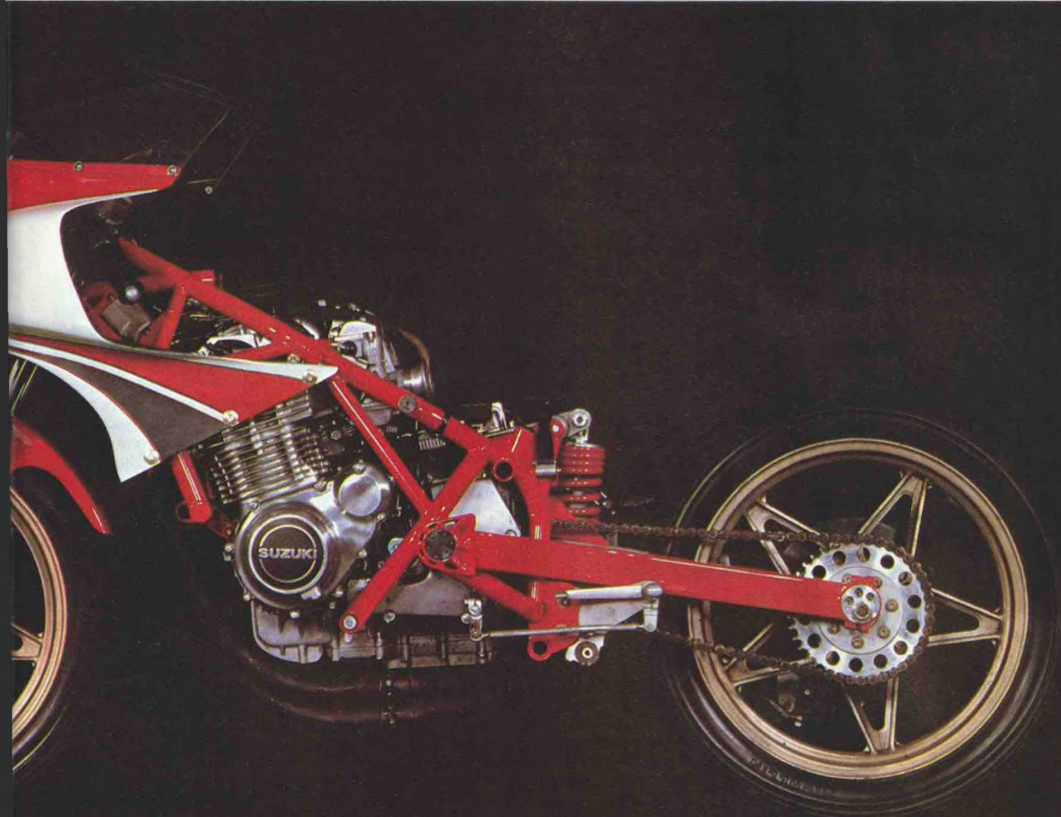
Bottom of shock attaches directly to swing arm; the top is linked to it through an aluminum rocker arm.
