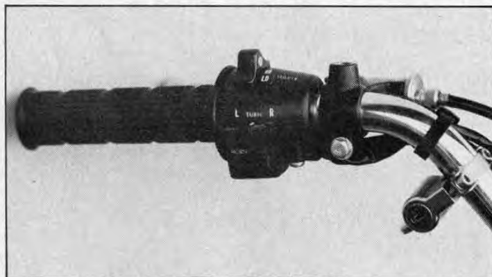
The KZ750 has good controls, hard grips and an easily-thwarted helmet lock.
