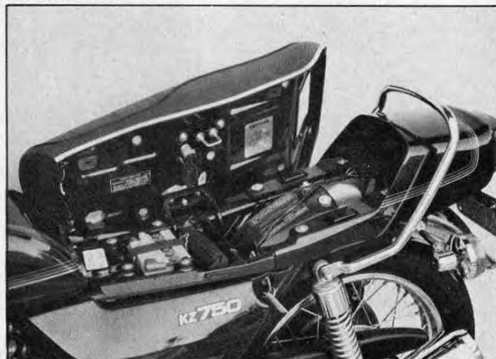
Lifting the locking seat reveals the air cleaner, battery, toolkit and tail-section storage.
