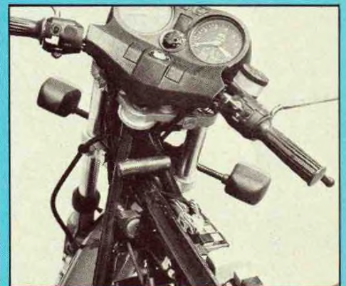
Designers are proud of the unitized console for instruments and steering head cover. Note neat wiring grouped on the right side of frame backbone.
