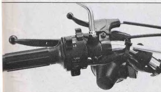
Short lever in front of clutch lever opens exhaust valves during compression stroke. Lever clicks off and piston is in the right position for easy one-kick starts.
