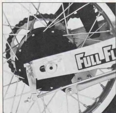
DR's Full Floater uses the same hub (we swapped while a tire was being fixed) but the swing arm is aluminum and longer.
