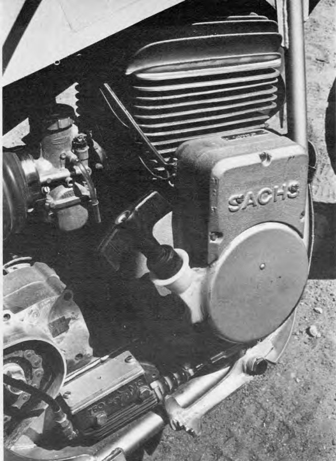
Right hand view of the engine clearly shows the pull-cord starter and the rear brake pedal which pivots from the front and is connected to the Kelsey Hayes master cylinder by an adjustable rod.
