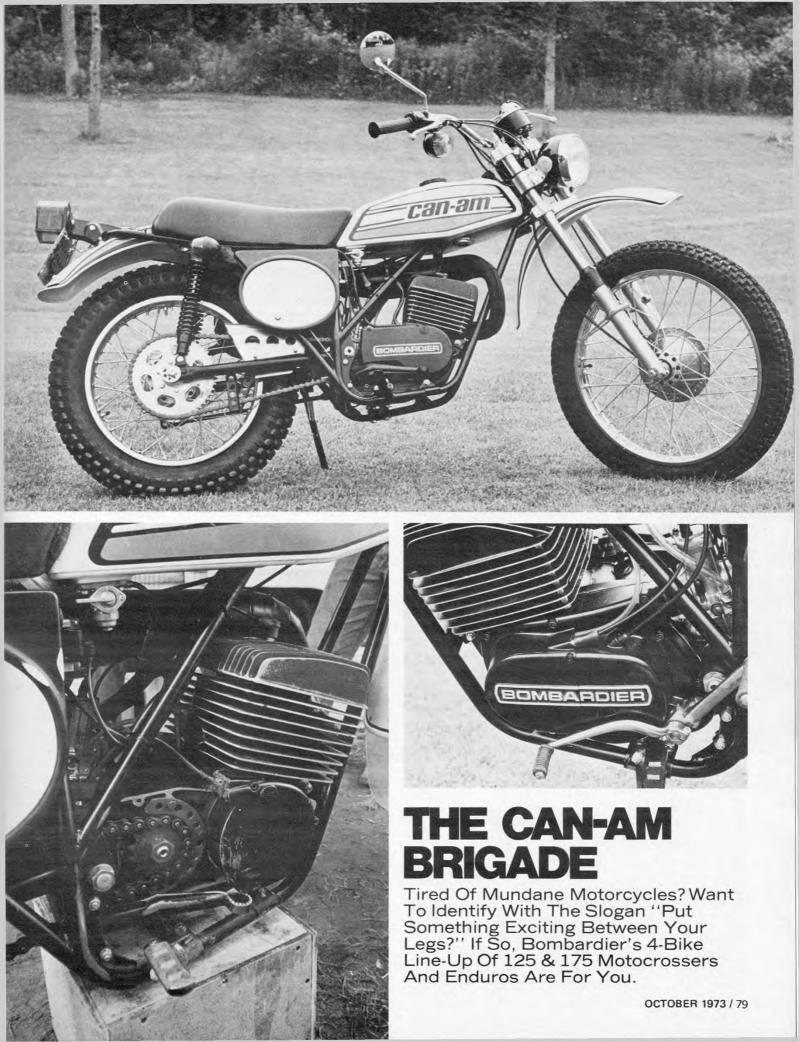
gears with a 3.286 reduction, to a six-plate wet clutch—which seems to stick a lot. From there it goes through a transmission which many have seen before. The six-speed unit is the same as the transmission on a KTM/Penton 175. Rotax, Bombardier's engine division in Austria, makes the unit for KTM. A sturdy chain guide around the output sprocket should eliminate broken cases from chainwhip.
