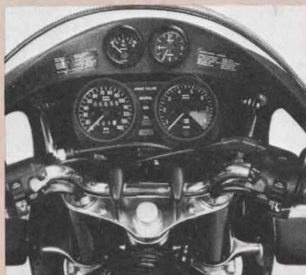
High-beam and turn-indicator switches are new and easier to use; steering damper remains only on the R100RS.
