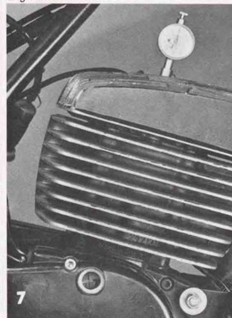
7 Can-Am 250 T'NT: Utilizing a dial indicator, the flywheel and reference marks should align at 1.4mm BTDC.
