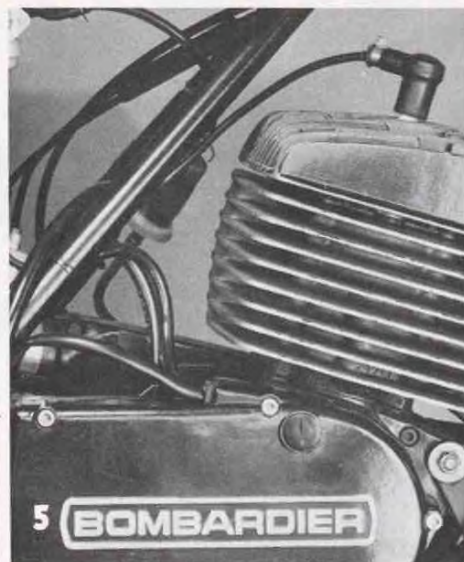
5 Can-Am 250 T'NT: A removable plug in the case makes for the easiest possible timing inspection.
