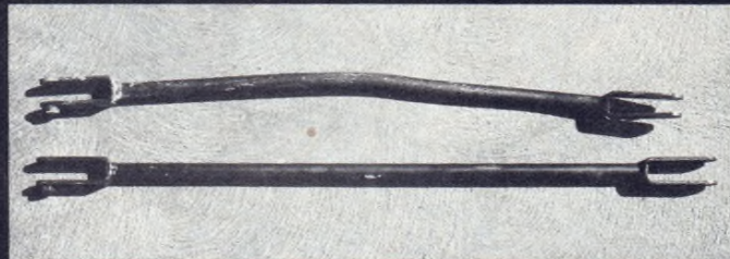
The brake anchor arm on top displays numerous encounters with rocks and other elements. It is replaced by the longer arm below.
