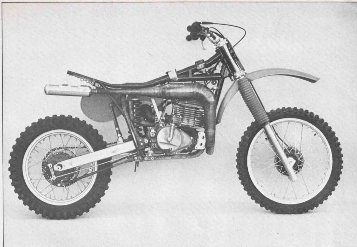
Frame has heavy-duty backbone. Pipe is handmade.
