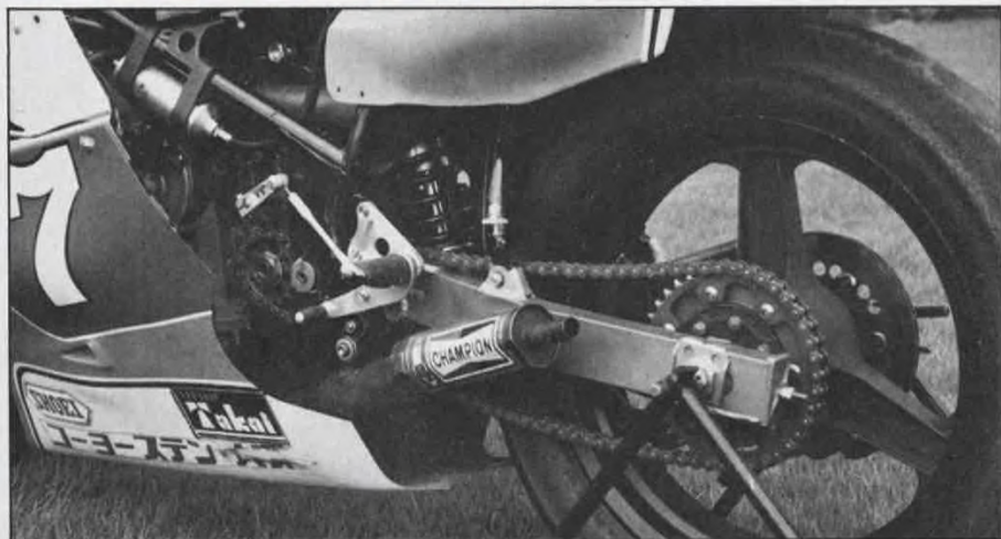
The Suzuki Floating Suspension System uses a large, almost-vertically-mounted shock connected to the swing arm at the bottom and to a rocker arm at the top, the other end of the rocker connecting about mid-way down the swing arm via struts. Note the remote oil reservoir for the shock, strapped to the frame below the gas tank.
