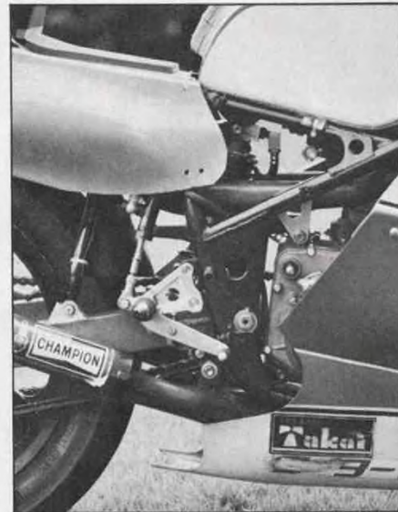
The upper end of the shock is visible in this view, along with the fitting for the remote reservoir. Shock body is mounted up. Suzuki officials would not allow photos with seat and tank removed.
