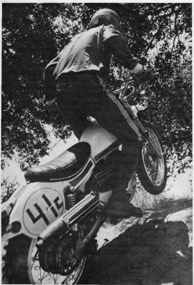
The units made it difficult, if not downright dangerous, to ride at a fast clip over rough ground. As a result, we had to be content with a fairly moderate pace for most of the event. With the progressive rate shock springs in the stiffest position and a 145-lb. rider aboard, bottoming was sometimes so severe that wheel lockup would occur when the tire lugs caught on the bolts that hold some of the fiberglass in place.
