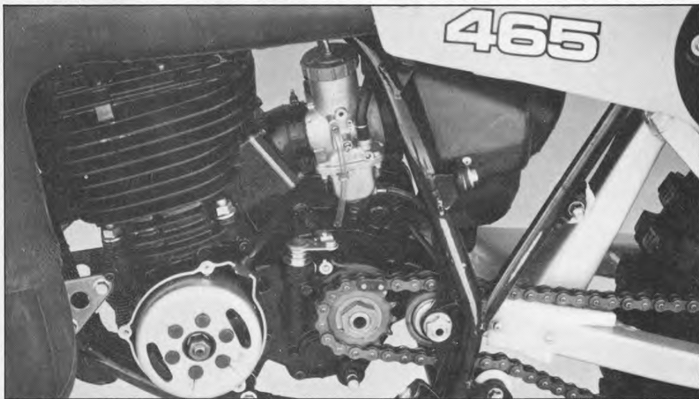
The 465 engine has an 85 x 82mm bore and stroke. Cases are extremely small and the swing arm bolt doubles as the rear engine bolt, eliminating the bracketry of years past. Ignition is CDI via an outside flywheel. Countershaft sprocket is close to swing arm pivot.
