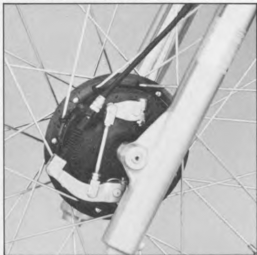
Front brake is a double leading shoe arrangement that retains the same hub as the F. Forks have 11.8 in. of travel and work beautifully.
