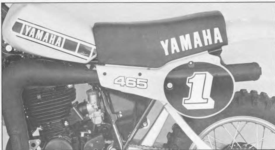
Seat height has been lowered despite the added suspension travel.
