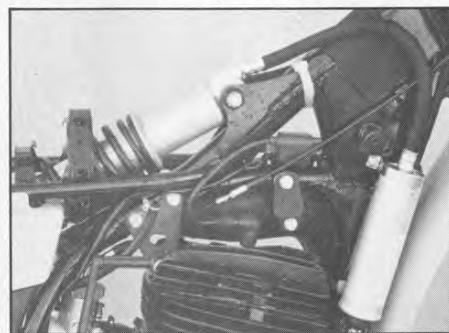
Aluminum bodied shock mounts half way back on the backbone tube. Reservoir is also aluminum and gas pressure can be adjusted.
