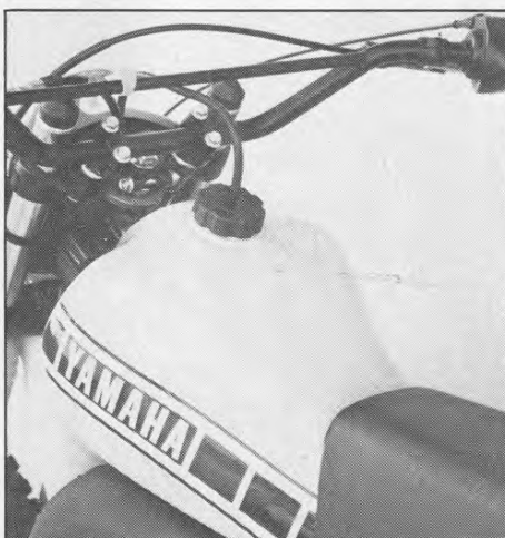
Plastic gas tank holds 2.4 gal. of premix and the decals don't fall off. Bars are correctly shaped and rubber mounted.
