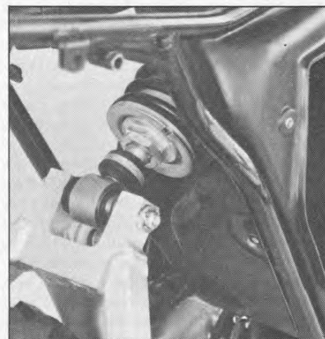
Shock rebound is easily adjusted by turning the finger knob. Spring preload is almost as easy but requires use of the supplied tool.
