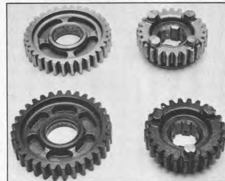
The GS1100's second gear is engaged when countershaft fifth's (right) three dogs slide into any three of six elongated oval holes in countershaft second (left). GS1000 parts (top) used four dogs into four longer holes. GS1100 system (bottom) engages faster, has less lash.
