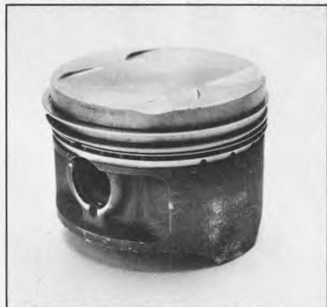
GS1100 piston has flat top, thin top ring, molybdenum disulfide on skirt to avoid scuffing during break-in.
