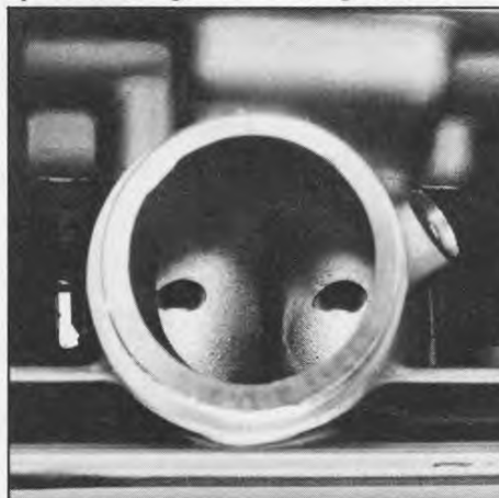
View down intake port shows that valve guides don't protrude very far into the port.
