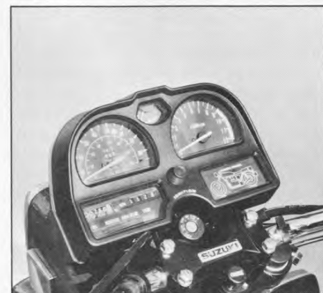
Instrument panel includes check panel with warning lights for head and taillight, brake fluid and battery acid levels.
