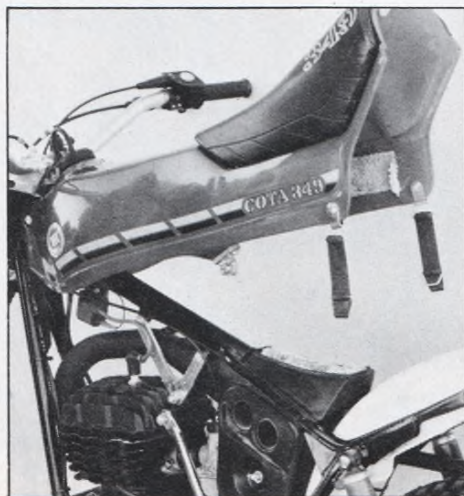
Lift-up Loplene seat/tank combination is convenient for servicing the Cota.
