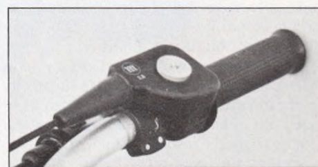
Straight-pull throttle works well when new, but is easily damaged in minor spills.
