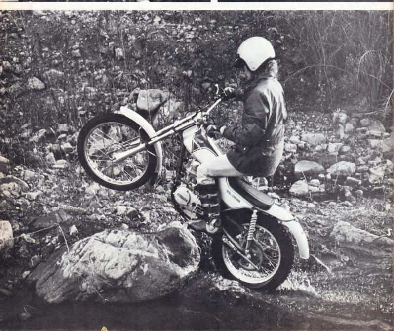
are right on. A nice feature on the shocks is the nylon strips glued to the shock bodies to prevent wear by the action of the springs. Shocks mount to the frame with flush Phillips-head screws, eliminating the possible danger of a rider smacking his leg into protruding bolts as he dabs in a section.
