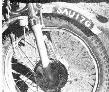
This shot of the rim of Englishman Scott Ellis' Puch 175 shows how tough six days of off-road riding is.
