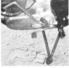
Awkward appearing kick arm works easily as does shift lever. Foot peg is mud free and grasps boot well. Side stand is nice.
