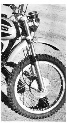
The front forks were a little soft in spring tension. Damping is good. Speedo cable should be attached to fork leg.
