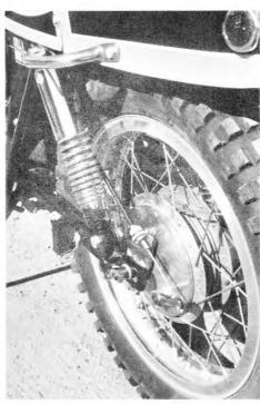
The Betor rear shocks with the chromed progressive wound springs have excellent spring strength and damping.
