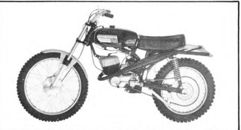
formed in huge presses, matched together and welded at the seams with automatic machines. All of this requires very little manpower. The engines are usually *hung* from the mounting tabs of the frame and add As with many European factories, the Italian made H-D Baja use the tubular backbone chassis. Note the large diameter backbone tube. Engine may or may not be used as structural member.
