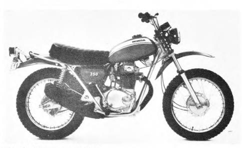
This dual purpose oriented Honda has a high center of gravity due to the location of the top heavy engine. Center of crankshaft is over two inches above axle height.
