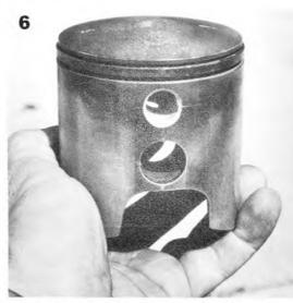
This hole provides the necessary path from the case to the special port located under the transfer opening in the liner.
