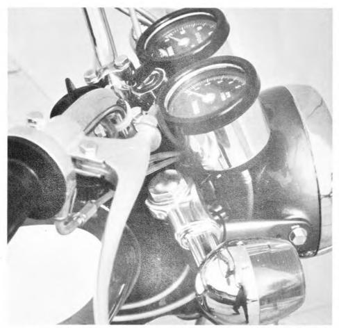
The front end of the bike looks busy. Along side of the headlight are the turn indicators. Between the speedo and tach is the ignition
