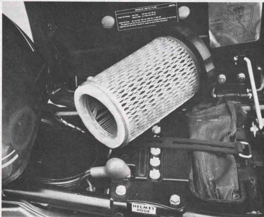
To replace the cartridge-type air filter element, raise the seat and twist the element out.
