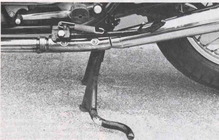
The centerstand foot bar grounds on hard left-handers, often making the rear of the bike skitter around.
