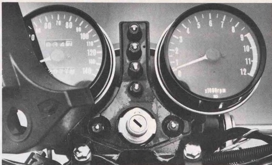
Replacing the idiot-light bulbs is simple. Just unscrew the plastic ring around the ignition switch and pop the light cover off.
