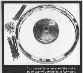
to replace your own wheel, or replace a bent rim, or substitute an alloy and / or a larger rim on your hub) by following this sequence. If you are installing a larger diameter rim, you'll need longer spokes. Notice that the spokes at the top of the photo have their heads angled at approximately 70 degrees from the shank of the spoke, and the bottom spokes have their heads angled at approximately 110 degrees.
