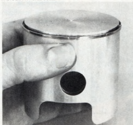
Flat top piston has less surface area to get hot as compared to a domed piston so the engine runs cooler.
